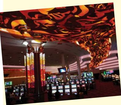
An undulating ceiling and lighting feature called "The River," completed in 2011, twists and turns above casino patrons on the gaming floor to give a cohesive, dramatic look. Made up of more than 30,000 electronic LED lights, it can produce any shade on the color wheel and can be changed to meet casino needs.
